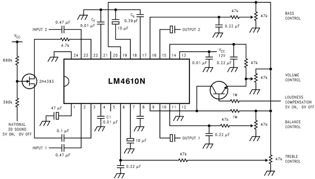
FIGURE 16. Application Circuit with Electronic Switching
