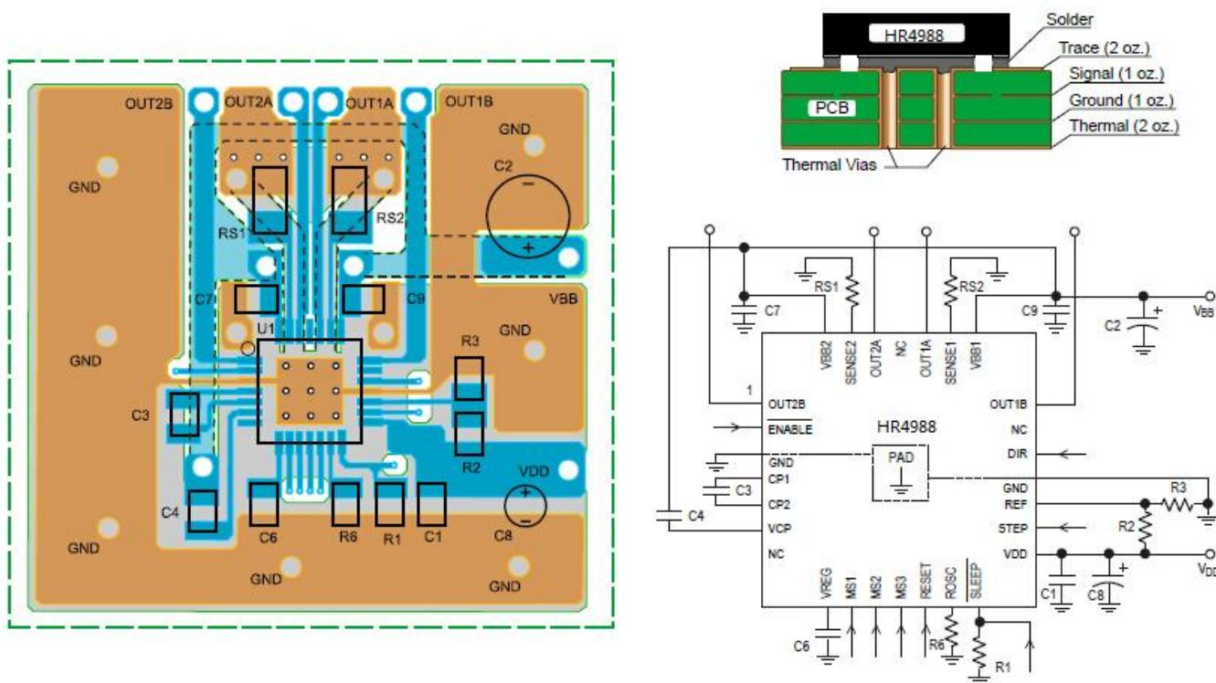
Figure 8: Typical Application and Circuit Layout
