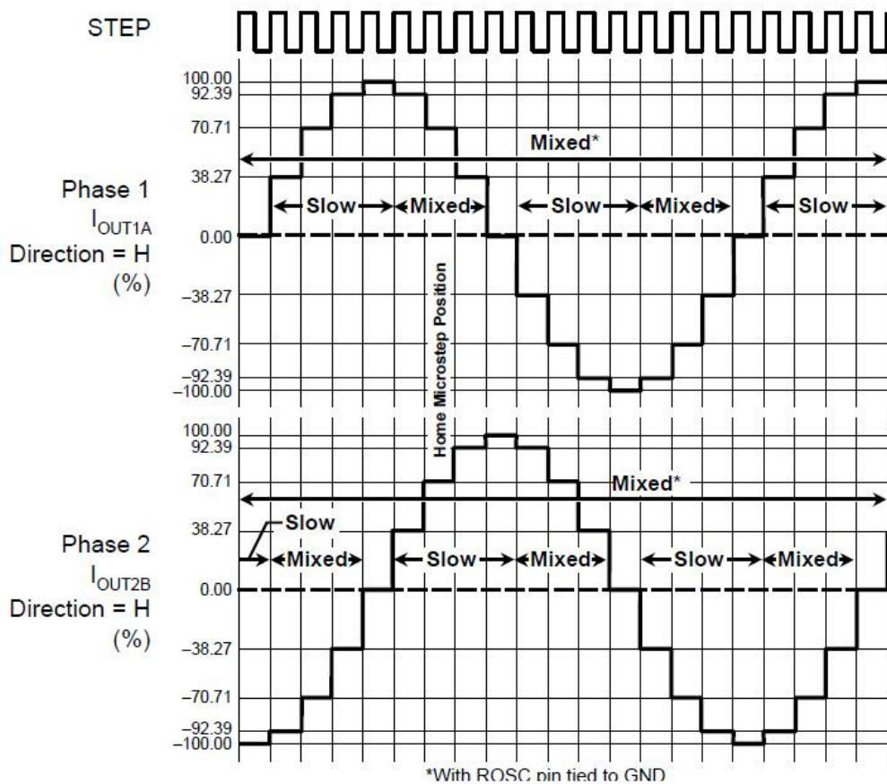
Figure 11: Decay Modes for Quarter-Step Increments
